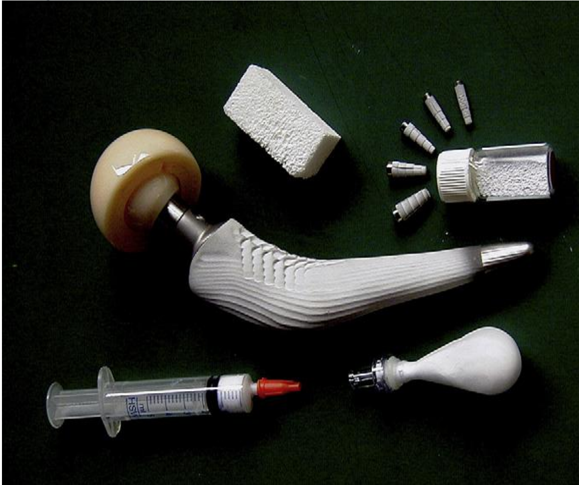
Several examples of commercial calcium orthophosphate-based bioceramics
